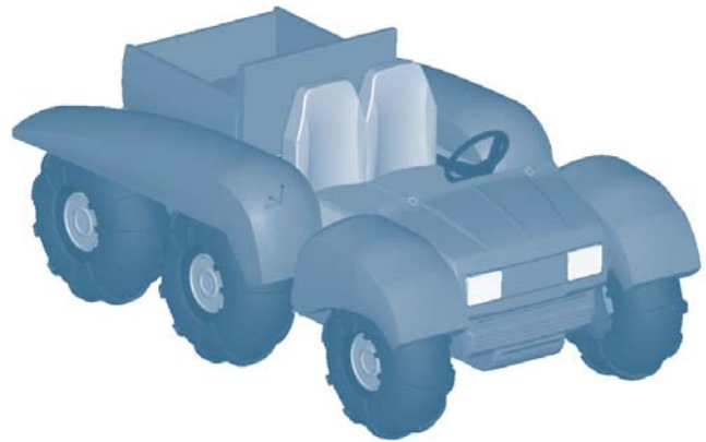
Amphibious Gator Utility Vehicle designed and rendered in Pro/ENGINEER by the student engineering teams.
